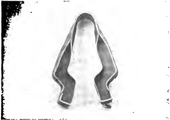
FIG. 1.—C-46-O Krupp steel chassis frame cross member. Closed on itself without showing cracks. Under shock test this steel deformed 3.03" after the fifth blow under standard conditions and the "proof" was then bent double, without showing cracks.
